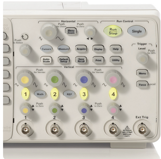
Figure 33. Oscilloscope front panels should include knobs for all key setup variables.
