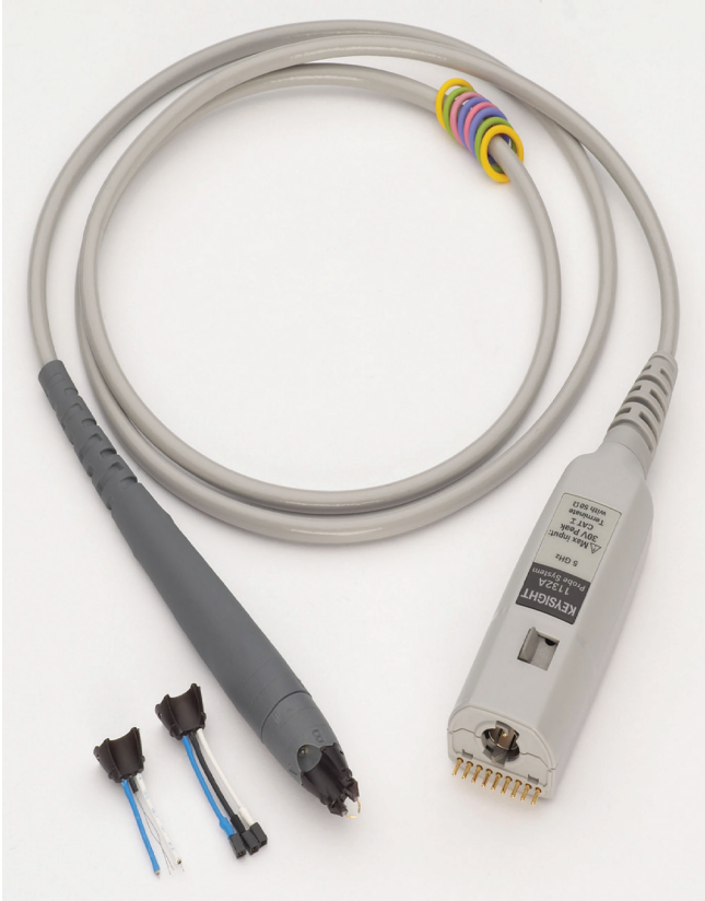
Figure 32. Keysight's InfiniiMode Series differential active probe.
